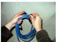
Once you're finished with all of the loops, use a Velcro cable lock to keep it all from uncoiling.
