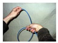
Start with the male XLR connector in your left hand and make a clockwise loop of the cable with your right hand.
