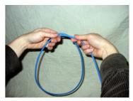
Make a full circle and catch the cable in your left hand to complete the "over" loop.
