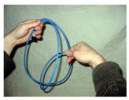
Bring this new loop under the front edge of the newly forming coil.
